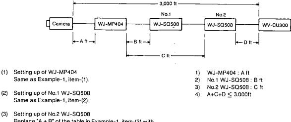
3) Setting up of No.2 WJ-SQ508 Replace "A + B" of the table in Example-1, item-(2) with the "A + C + D" of the diagram above. Note:
