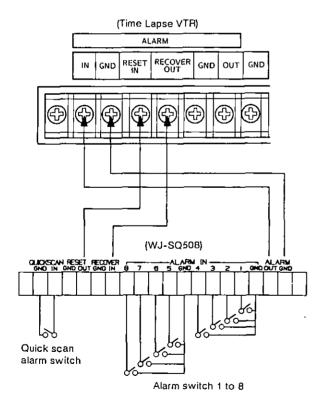
When the alarm time of the Time Lapse VTR is set shorter than the Sequential Switcher WJ-SQ508, the alarm mode of the Time Lapse VTR will be finished faster than the Sequential Switcher. At this time, the Time Lapse VTR will cease the alarm mode of the Sequential Switcher.
