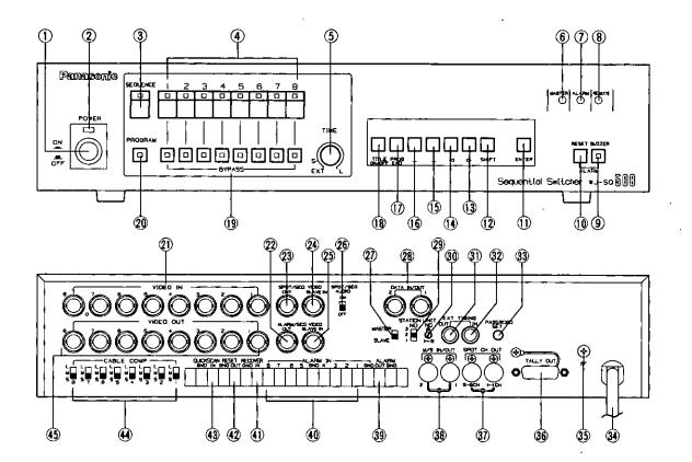
1. Power ON/OFF Switch (POWER ON/OFF) When this switch is depressed, the unit turns on and
