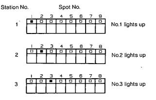
b. The Bypass LED shows the unit number as follows.
